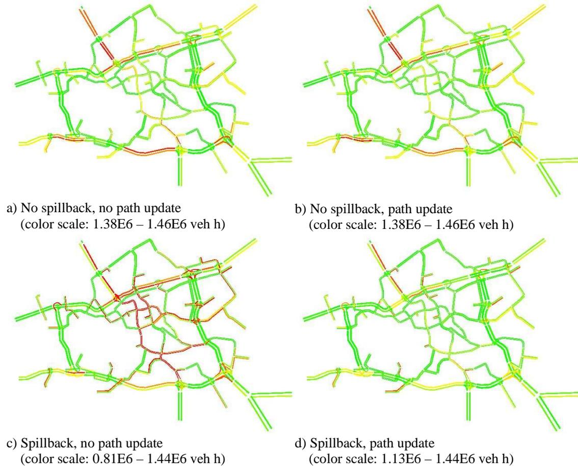
**Figure 5 The impact of blocking a link**
