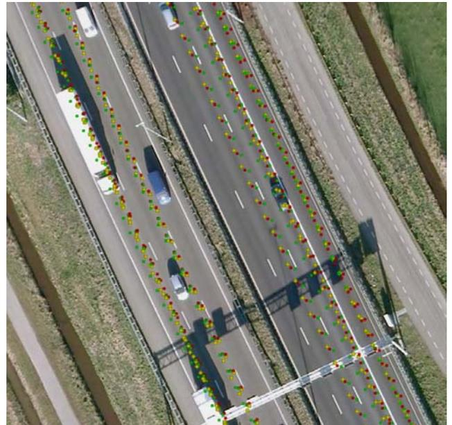
**Figure 5:** SF-PPP position trajectories overlaid on Google<sup>TM</sup> Earth image - results of u-blox TIM-LP receiver (green), Septentrio AsteRx1 receiver (red) and Trimble R7 receiver (yellow). The dots all show the correct lane. Note that on the North-bound stretch also the emergency lane has been used – the dynamic traffic management system allows to do so during rush hours (as was session 3, see also Figure 1).
