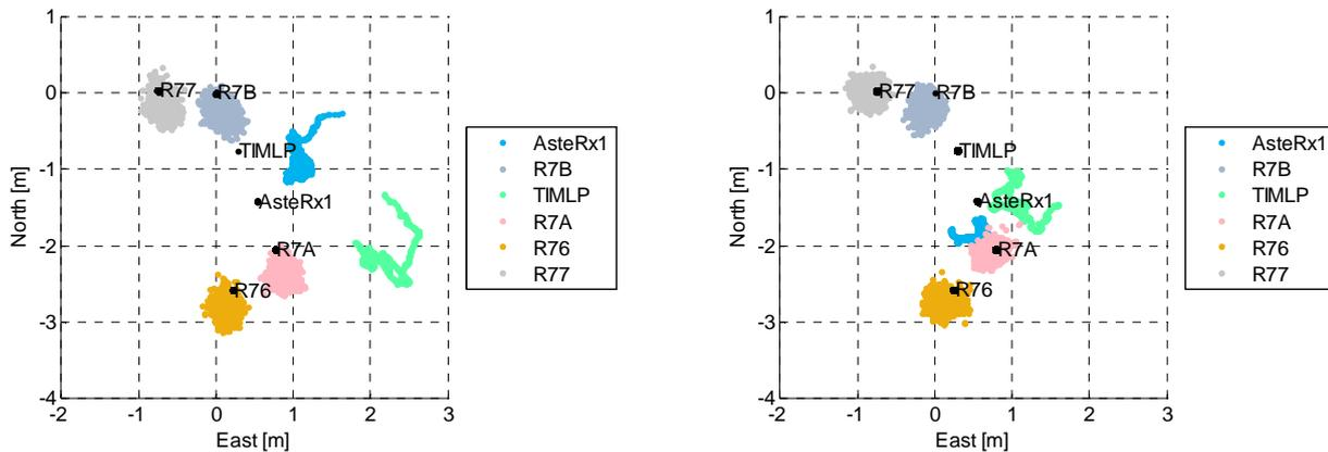
**Figure 8:** Static SF-PPP results for all receivers on the car, together with the ground truth positions (indicated by the black dots), for 5 minutes static part in session 2 (left) and session 3 (right). Horizontal positions in local East and North; the car is heading to the local South-East.
