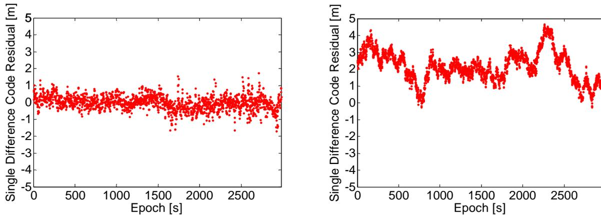
**Figure 9:** Single difference residuals of pseudorange measurements to satellite PRN18 for the baseline between the two Zephyr Geodetic antennas connected to Trimble R7 receivers at both ends of the wooden bar (left), and one of the Zephyr Geodetic antennas (Trimble R7) and the u-blox TIM LP with patch antenna (right); static part of session 2.
