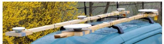
**Figure 3:** Antenna set-up on the roof of the test vehicle. In this paper only the antennas attached to the wooden bar at right are used. The ones at left (in the picture) are for a different experiment.
