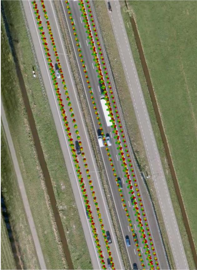
**Figure 6:** SF-PPP position trajectories overlaid on Google<sup>TM</sup> Earth image - results of u-blox TIM-LP receiver (green), Septentrio AsteRx1 receiver (red) and Trimble R7 receiver (yellow). The dots all show the correct lane. On the North-bound stretch this figure demonstrates a lane-change, to the far most left lane.
