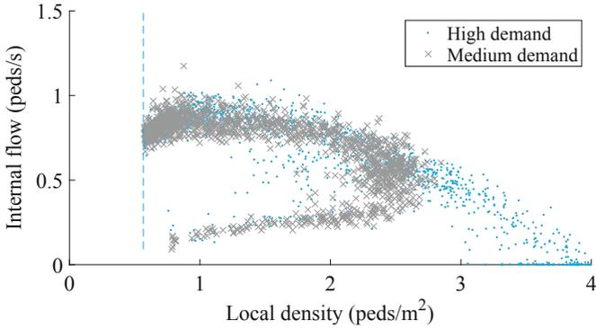
Fig. 5 Relation between internal flow and local density
