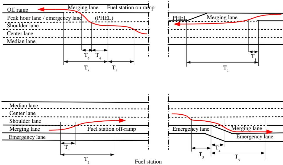
Fig. 4 The figure on the top shows the northbound and the lower figure is the southbound. The road stretch is longer in between the open areas in the middle (figure is not to scale);  $T_1$  to  $T_6$  are defined in Table 2. The red arrows indicate merging (right top and bottom left) and diverging (left top and bottom right) manoeuvres.
