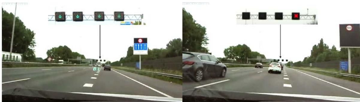
Fig. 2 Opened peak hour lane (left); Closed peak hour lane (right).
