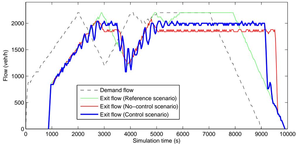
(a) Demand and exit flows over time in all scenarios. The demand flows are the flows measured by the detector located at  $x = 0.3$  km. The exit flows are the flows measured by the detector located at  $x = 29.9$  km. Flows are smoothed by using a simple moving average method: the flow for a given sampling period is the unweighted mean of the measured flow on that sampling period and the measured flows on the previous and next sampling period.
