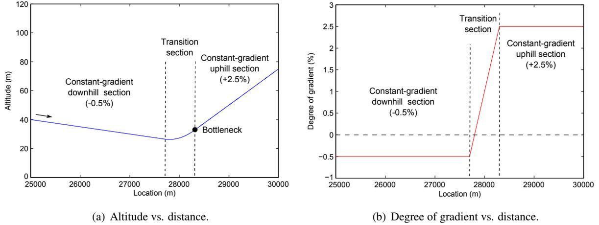
**FIGURE 2 Vertical alignment profile of the network (from  $x = 25.0$  km to  $x = 30.0$  km).**
