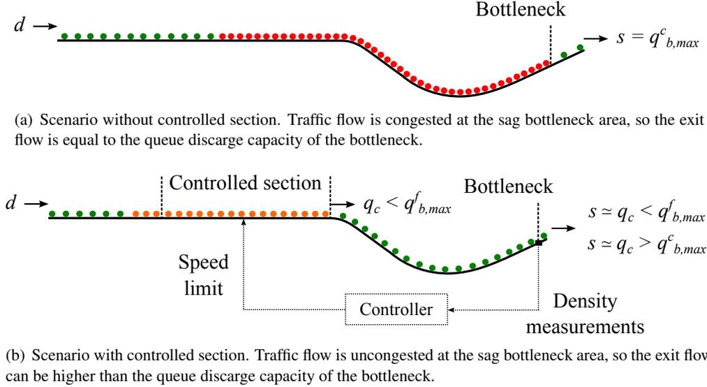
**FIGURE 1** Flows in the network ( $d$  is demand flow,  $s$  is exit flow,  $q_c$  is outflow from the controlled section,  $q_{b,max}^f$  is free flow capacity, and  $q_{b,max}^c$  is queue discharge capacity). Green circles represent vehicles in uncongested traffic conditions; red and orange circles represent vehicles in severe and less severe congested traffic conditions, respectively.
