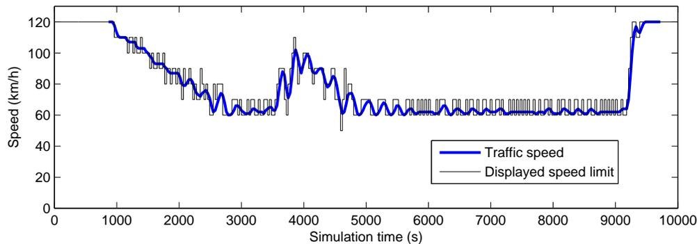
(b) Speed limit and average traffic speed over time at location  $x = 27.0$  km (i.e., 300 m before the end of the controlled section) in the control scenario. Traffic speeds are smoothed by using a simple moving average method: the speed for a given sampling period is the unweighted mean of the measured average speed on that sampling period and the measured average speeds on the previous and next sampling period.
