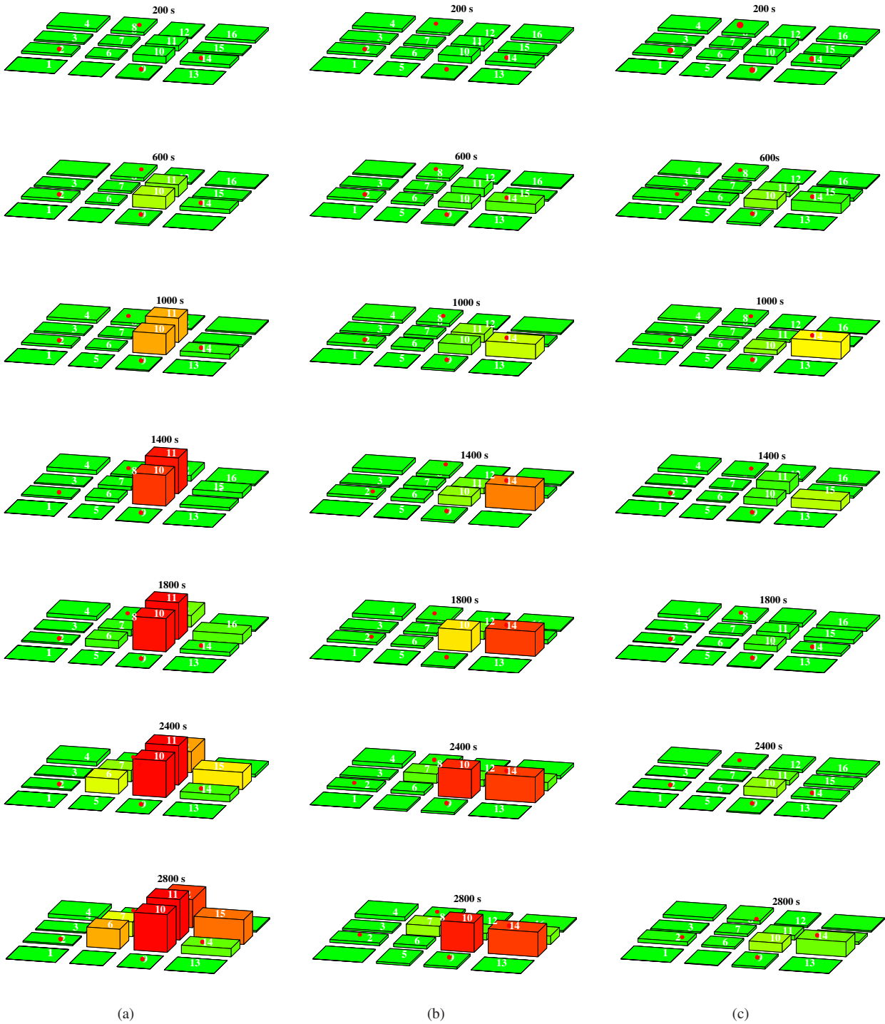
Fig. 5. Results for 4 \times 4 network, (a) Uncontrolled (fixed routes), (b) Shortest-path algorithm, (c) Optimal dynamic routing using MPC
