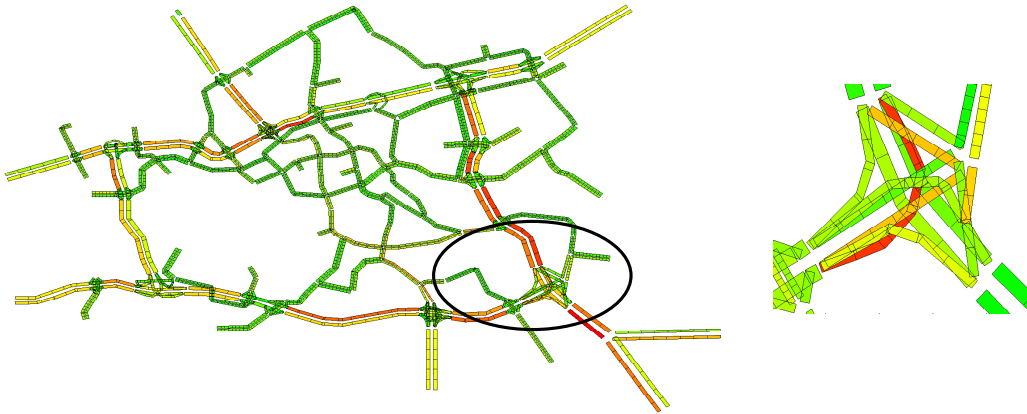
Figure 5 a) the impact of the blocking of a link b) the difference in link impact caused by spillback modeling
