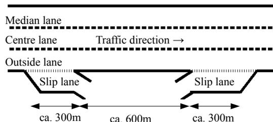
Fig. 3: The default design for motorway intersections
