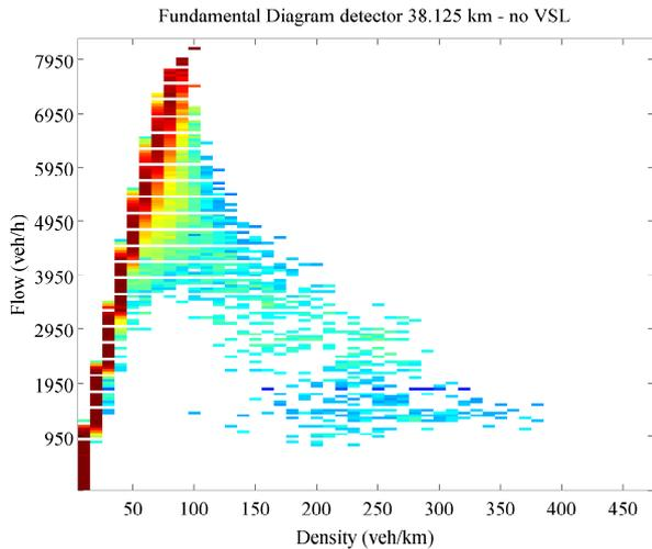
Fig. 4: Fundamental diagram in the flow-density plane
