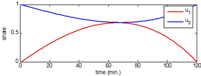
Figure 3 Dynamics of the optimal controls  $u_1$  and  $u_2$  for the two hour simulation period when the mean travel time is optimized.
