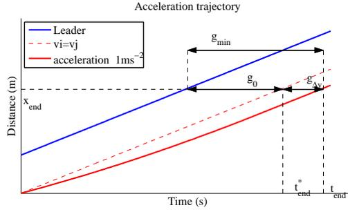
FIGURE 3 Illustration of the minimum gap
