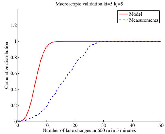
(b) Distribution of LCs in bin  $4 < k_i < 6$  (density in the origin lane) veh/km/lane and  $4 < k_j < 6$  (density in the target lane) veh/km/lane
