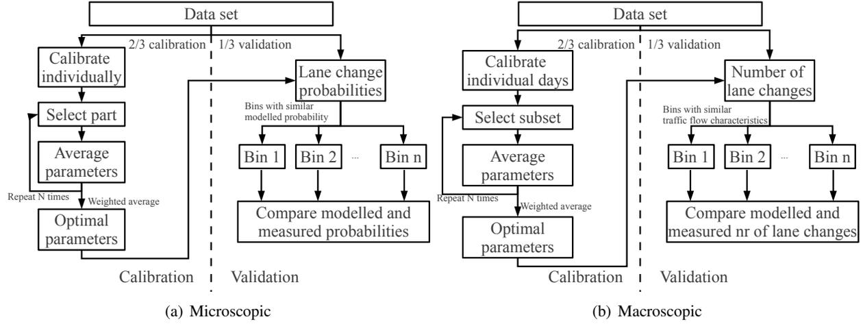
**FIGURE 4 An overview of the steps in calibration and validation**
