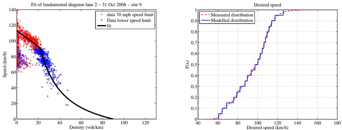
(a) The fundamental diagram in the speed-density plane for the middle lane for a one-minute aggregation time (b) The distribution of the desired speed and the modelled distribution
