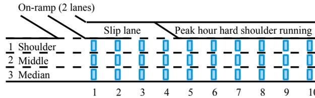
**FIGURE 1** The layout of the motorway and the detectors. The detectors are placed at approximately 100 meter distances. Note that in the United Kingdom, people drive at the left hand side of the road. That means, left to right in this figure. The next off ramp is 4.5 kms further downstream.
