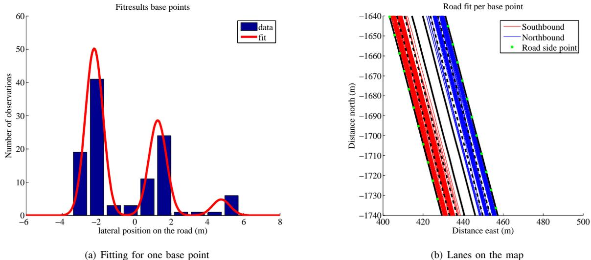
**Fig. 7: Finding the lanes: lanes based on the base points**
