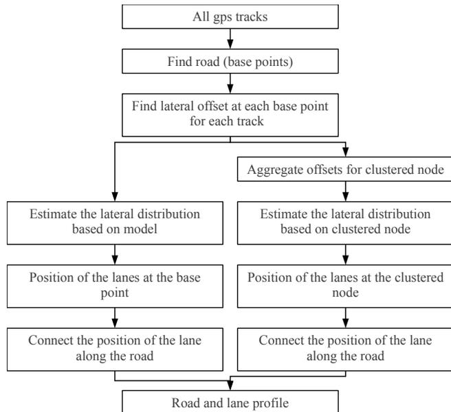
**Fig. 1:** An overview of the steps taken in the research. In the left branch, the position of the lane is based on measurements for each base point. In the right branch, the lateral passing positions are first combined into clustered nodes for an increased accuracy, and on this larger sample the lane positions are estimated.
