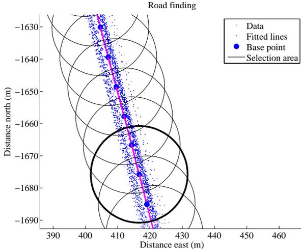
Fig. 5: The measured data points and the results of the process of finding the road points.
