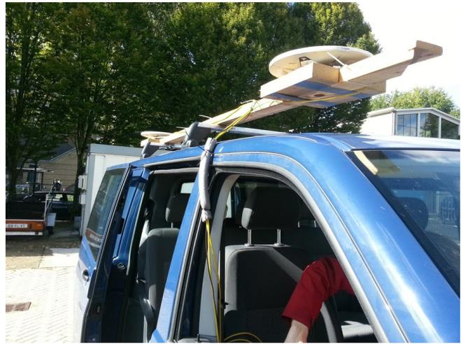
**Fig. 2:** The vehicle equipment used for the test; there are two D-GPS receivers for the ground truth and a PPP-GPS receiver in the middle.
