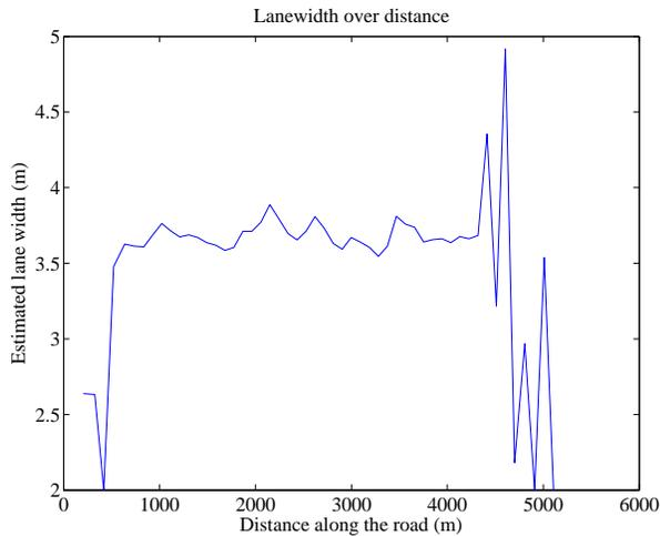
**Fig. 10: Estimated lane widths as function of distance (north-bound). Again, in the first 500m and after 4500m of distance, the test vehicle does not travel in the designated lanes, but is merging into, or out of the main road, so trajectories are not distributed over the lanes.**
