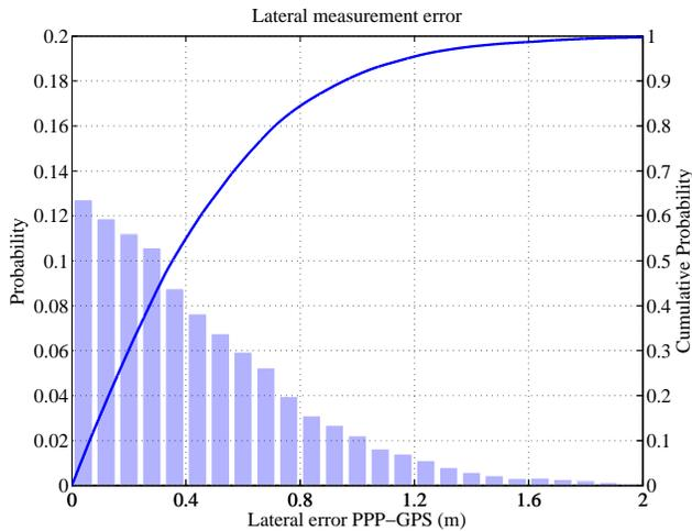
**Fig. 3: The histogram and the cumulative distribution of the errors in the PPP-GPS position lateral to the driving direction. The errors are constructed with a D-GPS as reference ground truth.**
