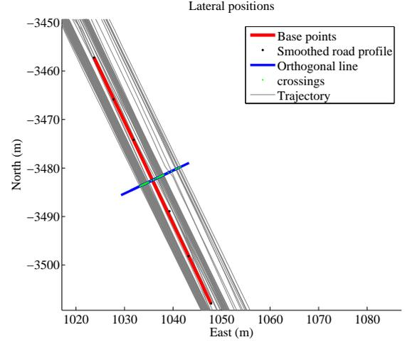
Fig. 6: The lateral positions are calculated by reconstructing where each of the trajectories crosses a line orthogonal to the (average) road direction
