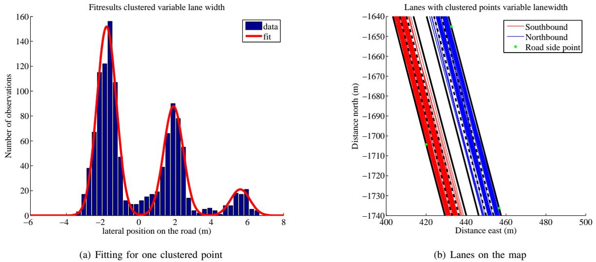
**Fig. 9: Finding the lanes: lanes based on the clustered points with a variable lane width**
